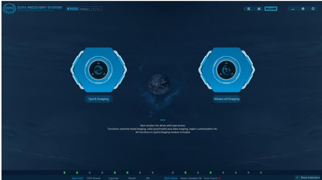
Select the target defective HDD as data source, set the imaging destination and continue to the imaging window.
